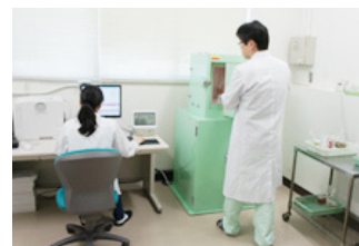
Analysis using a germanium semiconductor detector(2)
