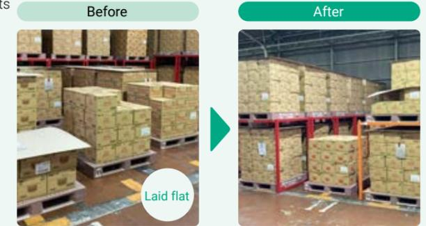
Utilizing space more effectively by switching from laid flat to steel pallets (Ueno Plant)
