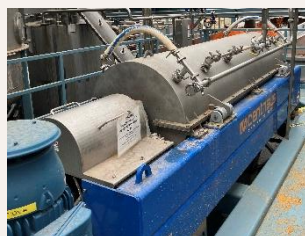
Centrifugal separator: Centrifugal separation allows for adjustment of fiber content, contributing to improved yield for Kagome Inc (secondary processing companies).
